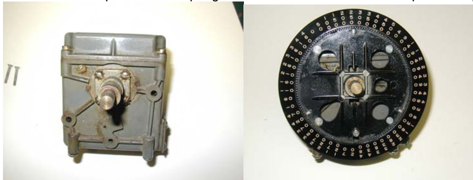
Then start reassembly by placing the number dial on the gear drive shaft with the 250 number at the 12:00 o'clock position. A very small amount of white grease can be placed on the gear and shaft area.
