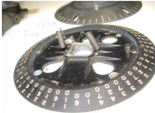
The spring position should be noted . If the spring is inverted the micrometer dial will bind.
